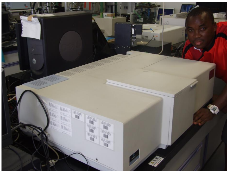
Fig. 8.1 Photo for UV/Vis/NIR spectrometer (Lambda 900, PerkinElmer).
