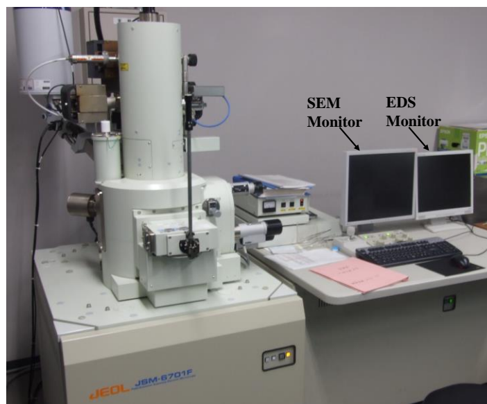
Fig. 3.7 Photo for FE-SEM (Field Emission Scanning Electron microscopy).
