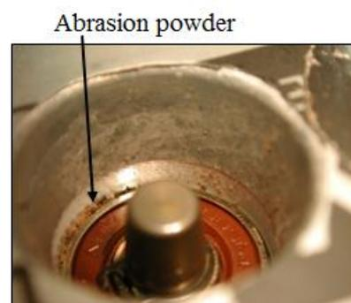
Fig3-7 Abrasion powder caused by fretting corrosion
