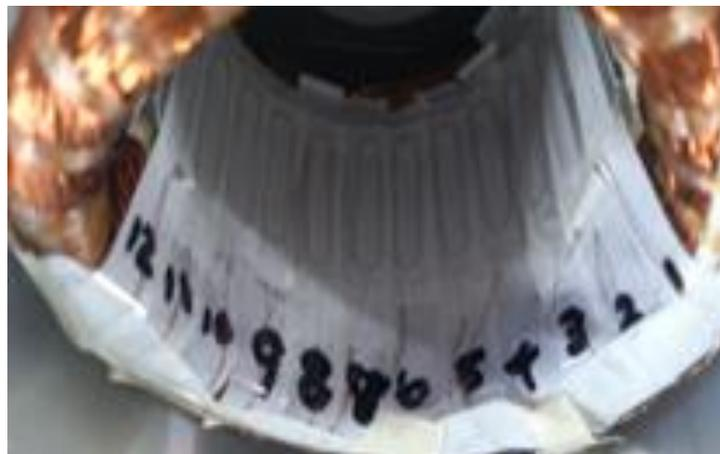
Fig.2-27 Enlarged view of search coil installed on stator teeth
