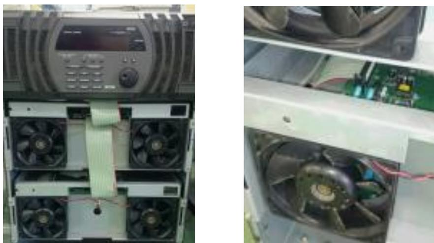
Fig.1-21 Fan motor installed on AC power source
