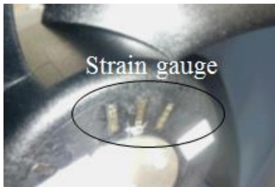
Fig.4-19 Strain gauge on impeller
