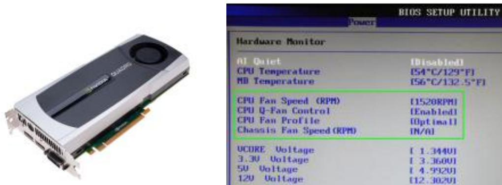
Fig.1-17 Fan motor speed control by BIOS
