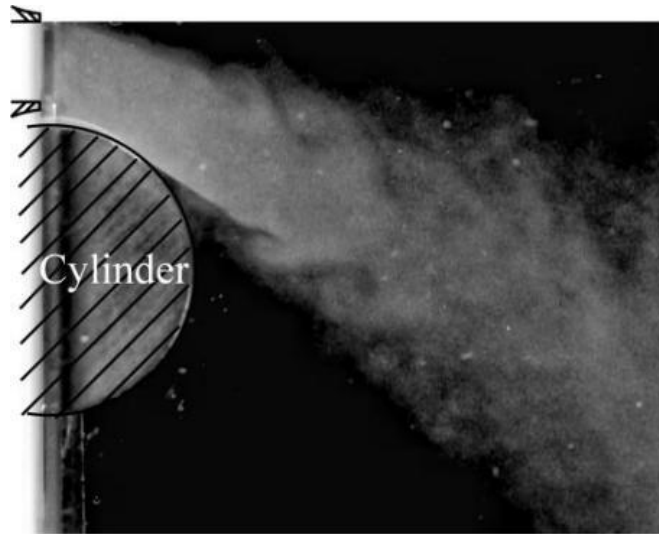
(a) Visualization observation. Photograph was taken at the frame rate of 960 Hz
