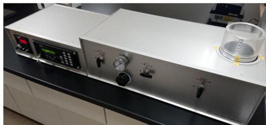
Fig. 2.3 Instrument for measuring flow resistance of porous materials.
