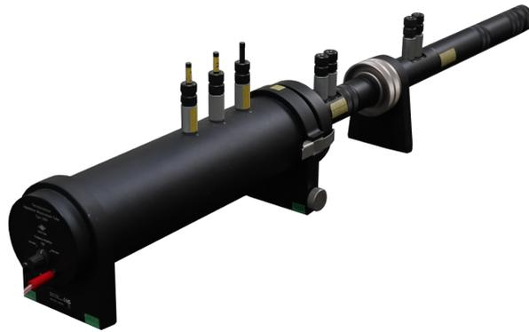
Fig. 2.2 Impedance tube for measuring sound absorption coefficient of  $\phi 29$  at normal incidence of 500-6400 Hz using Brüel&Kjær Type 4206T.
