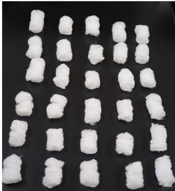
Fig. 2.4 Samples of fiber-based sound absorbing materials for sound absorption coefficient and microstructure analysis.
