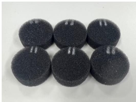
Fig. 2.7 Experimental samples of polyurethane foam.
