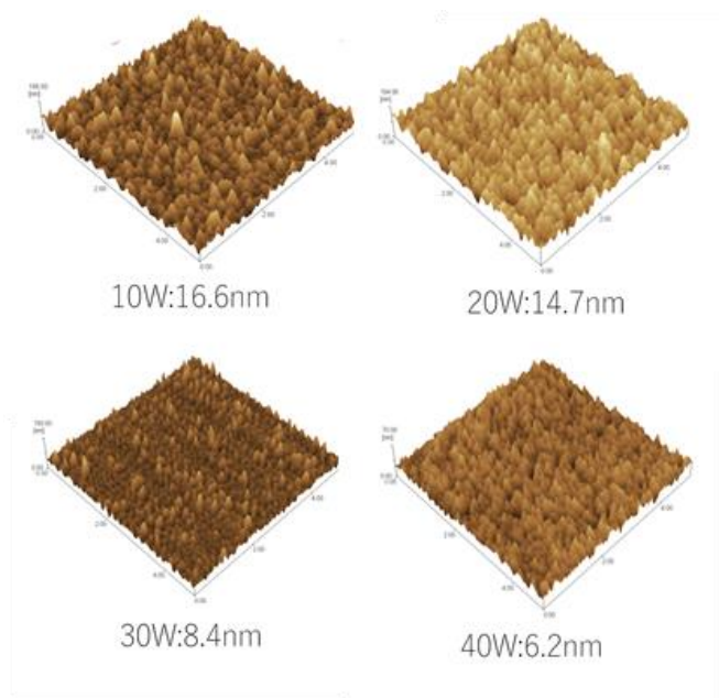
Figure 4.3 Surface morphology and surface roughness (Ra) for copper oxide films fabricated under various sputtering powers.
