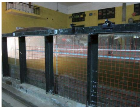
Fig. 1 Water surface in flume, case study with discharge Q=0.045(\text{m}^3/\text{s}) .
