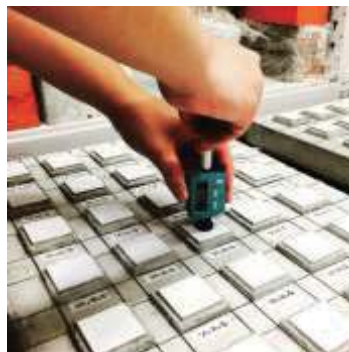
Fig. 2 Image of non-destructive hammering test (HLD)
