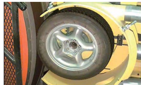
Fig. 2 Drum type tire wear tester
