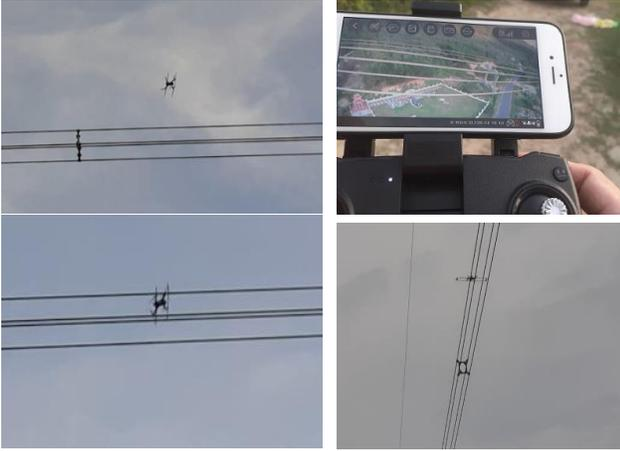
Figure 9. Experiment of drone parked on the power wire 500kV
