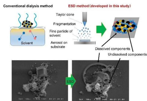
Figure 1 Schematic of electro-spray dialysis method
