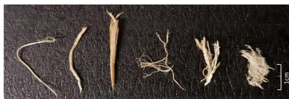
Fig. 6. An example of different shape of EFB fiber
