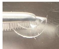
Fig. 1. Appearance of polyether/SL gel electrolyte.
