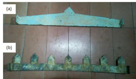
Figure 2. (a) Nose shape blade, (b) comb shape blade
