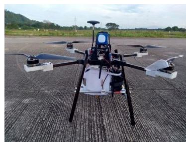
Fig. 1. The Unmanned Aerial Vehicle (UAV) Pesticide Sprayer Assembly
