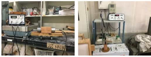
Fig 1. Ultrasonic propagation velocity measuring instrument (left)
