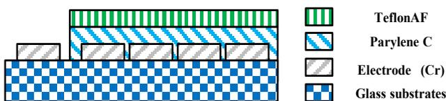
Fig. 9 Cross section of the one-plate EWOD device
