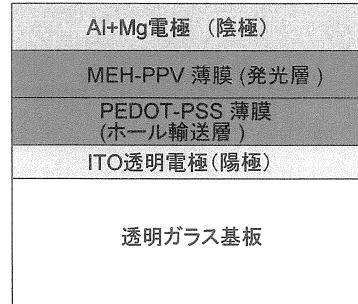
Fig.5 Structure of OLED
