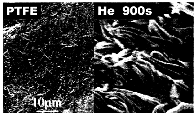
Fig.3 Surface morphologies of PTFE un-irradiated and irradiated by He^+ ion beam
