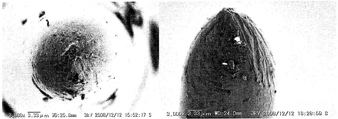
Fig.5 Fracture surface of Al bonding wire ( $\sigma_{\max}=321 \text{ MPa}$ ,  $N=6.14 \times 10^4$ ,  $El=21 \mu \text{m}$ )
