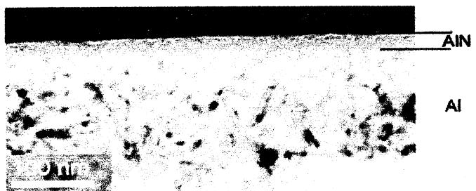
Fig. 2. Cross-sectional TEM image of (111)Al substrate with nitridation. AlN layer thickness is approximately 20 nm.
