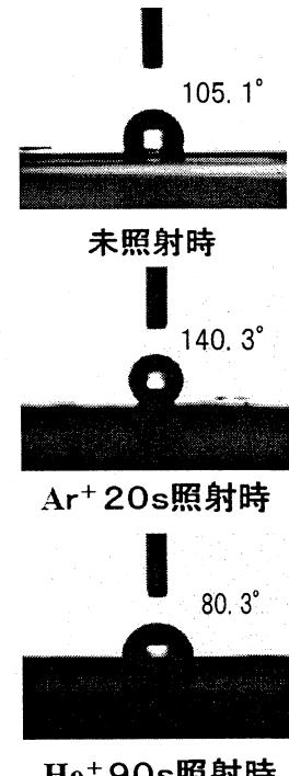
Fig.4 Photographs of contact angle measurement
