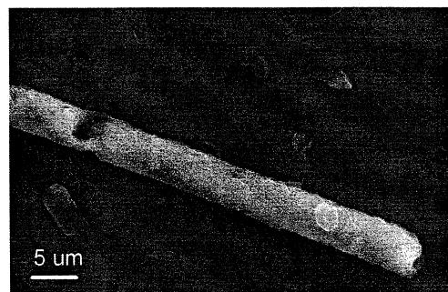
Fig.3: SEM images of anthracene deposited by RESS method at  $25\text{ MPa}$ ,  $100^\circ\text{C}$ . (upper: central part of deposition, lower: rod-type shape)
