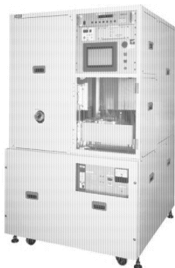
Fig. 15 ICP etching system installed last year at Kogakuin University.
