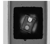
**Fig. 13** GaN-based LED installed in Si micro-cup with certain twist angle.
